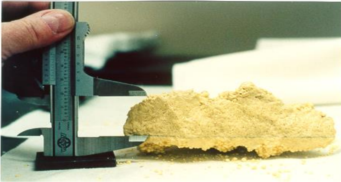
Photo #3 Caking of sulphur on surface of cargo
